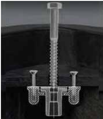
Non-Seizing Bolt System Allows Field Replacement
